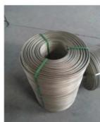
Calcium metal or metallic calcium is a silver–white metal. It is mainly used as a deoxidizing, decarburizing, and desulfurizing agent in alloy steel and special steel production. It is also used as a reducing agent in high–purity rare earth metal processes.
